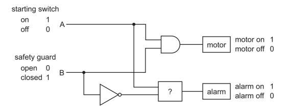
The circuit must only allow the motor to start when the safety guard is closed. If the safety guard is not closed when the starting switch is on, the alarm must sound.
